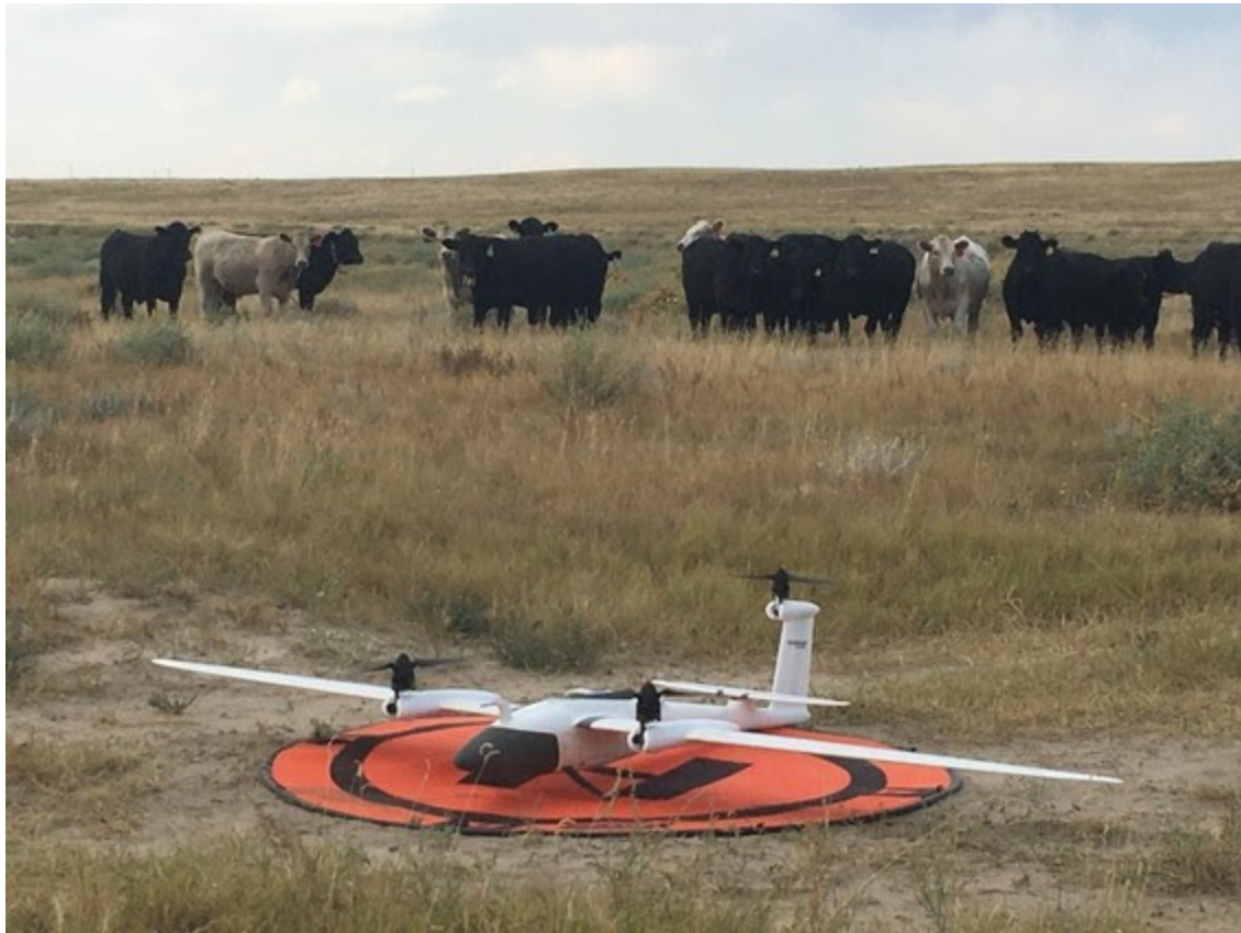
Figure 2. Cattle observing the UAS system used to acquire imagery for the study. The vertical take-off and landing capability and fixed-wing design allowed efficient image acquisition over large areas, resulting in a very large dataset requiring SCINet resources for processing.
